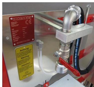
Outlets for resin and catalyst
