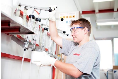
Wall Dosing Units
